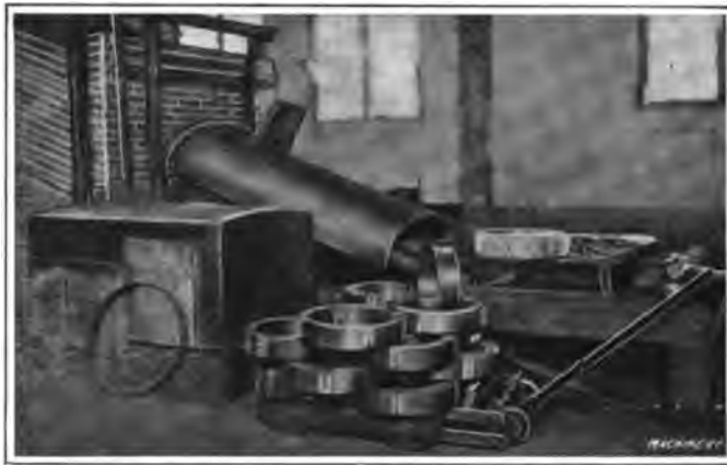
Fig. 14. Entering End of Gas Medium Furnace for Annealing Steel
